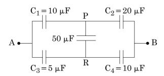
Calculate the equivalent capacitance between points A and B in the circuit below. If a battery of 10 V is connected across A and B, calculate the charge drawn from the battery by the circuit.
